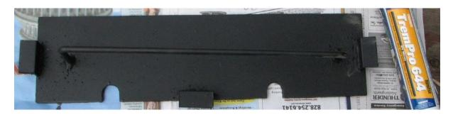
Run a bead of silicone all around the edge (1) and then run a thick bead on top, right near the edge (2) (See photo below)
