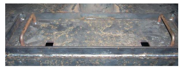
This cover MUST be sealed with standard, readily available RTV (Room Temperature
